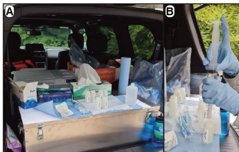
Fig. 1. (A) Water filtration in a mobile field laboratory set up in the back of a vehicle using (B) GSC water filtration and collection protocols developed by Hall (1998).
