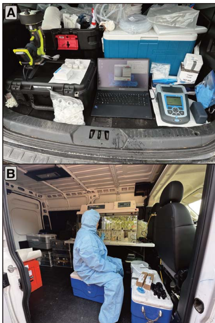
Fig. 6. (a) Field set up for rapid field analysis using a portable pXRF and spectrophotometer in the back of a vehicle, (b) water samples processed for ultrafiltration in a mobile laboratory set up in the back of a minivan.
