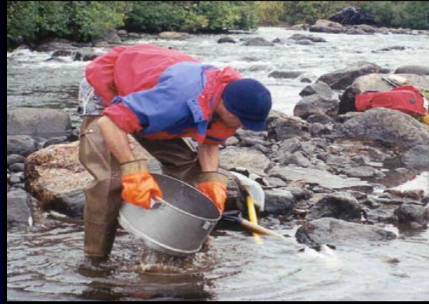
2. Wet Sieve -2mm fraction, coarse discarded
