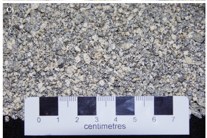
Fig. 8. A) Sample site of the unconsolidated weathered Silurian-Devonian granite (grus) used for GSC blank heavy mineral samples. B) Close-up view of the blank sample material. C) Close-up view of the 2–4 mm fraction of the blank material.
