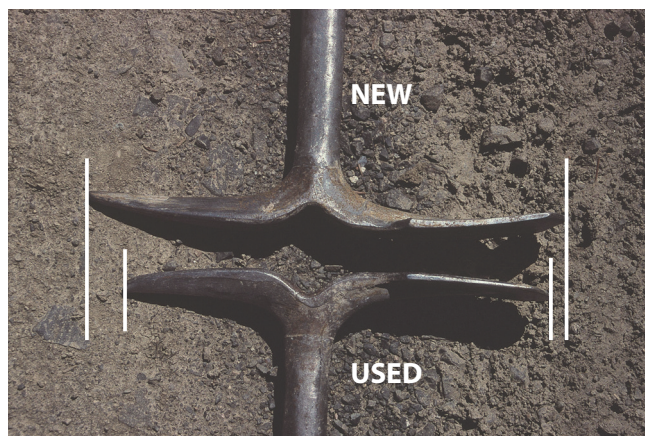
Fig. 1. Two hoe-picks of the same brand. The top one is nearly new and the bottom one has been used for three field seasons. Note that the old one has visibly lost metallic mass (distance between the white lines), which has, in part, ended up in sediment samples collected.
