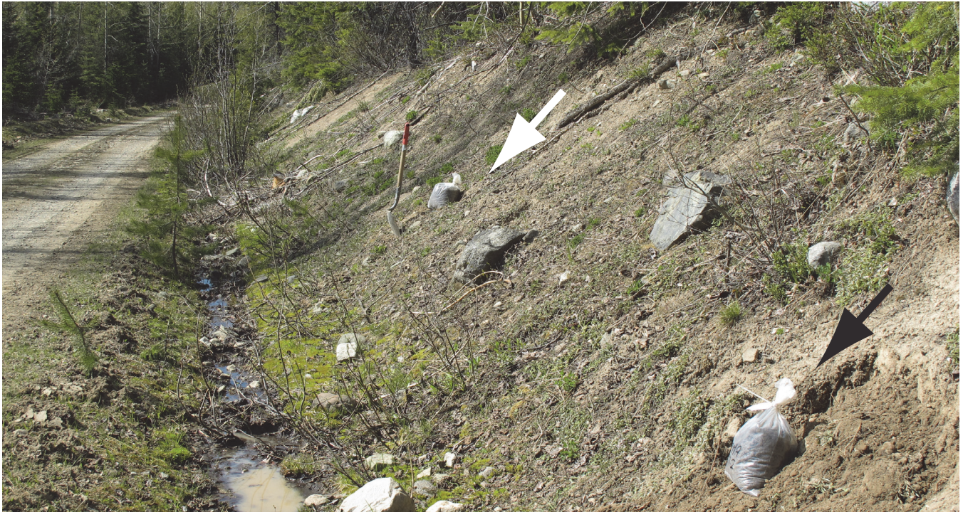
Fig. 7. Example of a till sampling site with a routine (black arrow) and field duplicate (white arrow) sample collected in the same sedimentary unit and at approximately the same depth.
