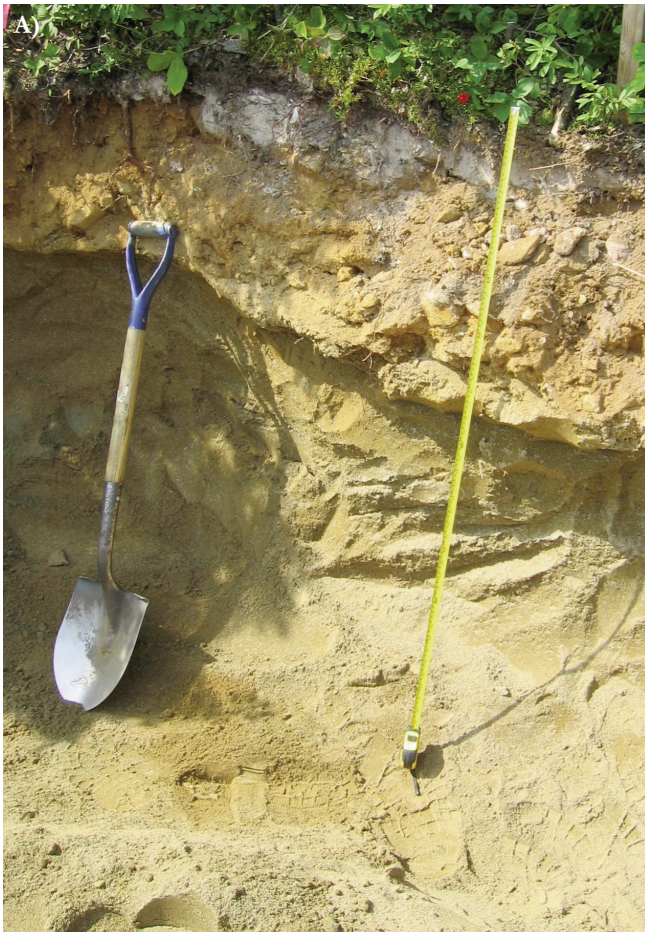
Fig. 8. A) Sample site of the unconsolidated weathered Silurian-Devonian granite (grus) used for GSC blank heavy mineral samples. B) Close-up view of the blank sample material. C) Close-up view of the 2–4 mm fraction of the blank material.
