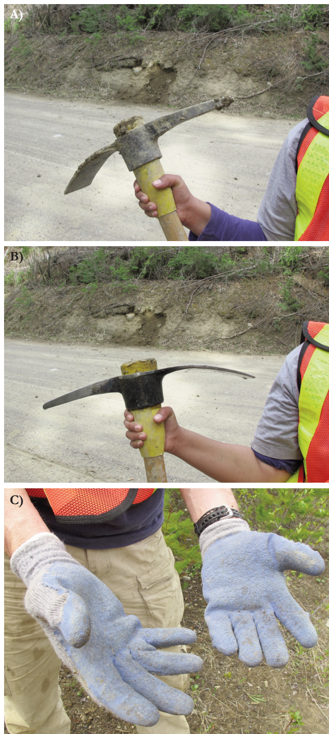
Fig. 4. A) A dirty pick with sediment stuck to it after the collection of a sample, and therefore unsuitable for the collection of the next sample. B) A cleaned pick ready for the collection of a sample. C) Work gloves represent a potential source of contamination.
