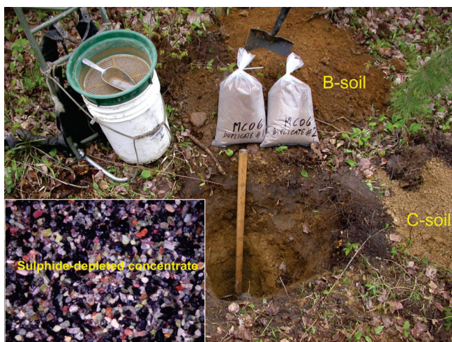
Fig. 5. Typical sample pit in oxidized till in Canada. Till excavated from the B- and C-horizons of the overprinted soil profile has been piled separately to illustrate their different oxidization states. Ideally, the sample is obtained from the weakly oxidized, pale yellow-ochre C-horizon below the highly oxidized, dark red-ochre B-horizon, generally at a depth of 0.5 to 1 m. The insert shows the heavy mineral fraction of the till in which most of the original sulphide grains have been consumed by oxidation.
