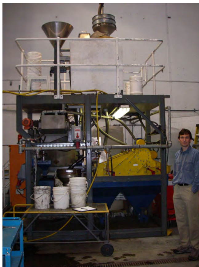
Fig. 4. Micro dense media separator used at Mineral Services Canada to separate kimberlite indicator minerals (photo from Mineral Services Canada).
