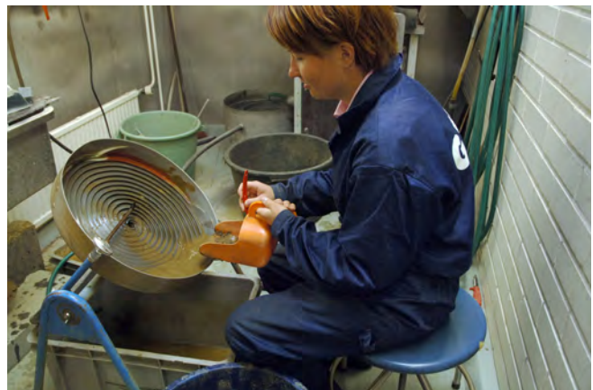
Fig. 6. Lab-based rotary spiral concentrator used by the Geological Survey of Finland (photo from P. Sarala, Geological Survey of Finland).
