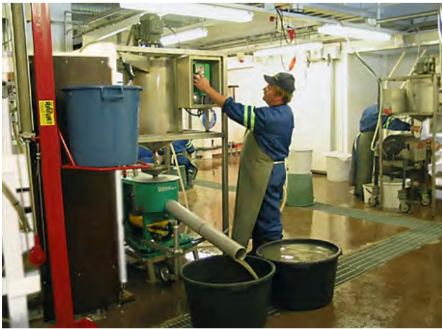
Fig. 5. Lab-based Knelson concentrator used to prepare a preconcentrate for recovery of kimberlite indicator minerals from till by the Geological Survey of Finland (from Marmo et al. 2008).
