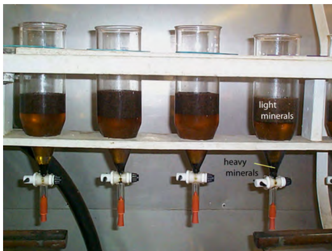
Fig. 7. Separation of heavy and light minerals is carried out using a specific heavy liquid of known density in separatory funnels. Heavy minerals sink and light minerals float to the top (photo from Overburden Drilling Management Ltd.).
