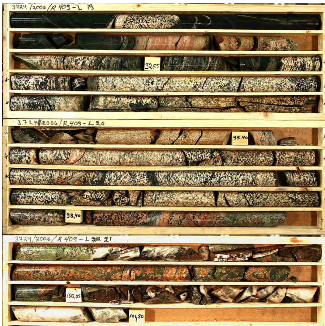
Fig. 6. An example of the drill core R409 from Petäjälehto. Drill core from 90 m to 101.80 m, which is composed of quartz–hematite–epidote breccia associated with the contact of a monzonite dyke.
