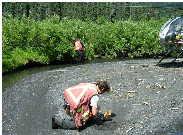
Fig. 1. Stream sediment and water collection during a helicopter-supported regional geochemical survey in northwestern British Columbia. One sampler is collecting sediment from a point bar that is sufficiently large enough to allow a field duplicate to be easily taken. The second sampler is taking a water sample and will record information about the site on a field form.
