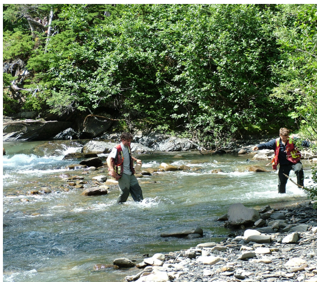
Fig. 2. Stream sediment sampling in a high-energy stream in northwestern British Columbia. The samplers are returning from what is clearly a difficult collection from a mid-stream bar. This site would be ideal for collecting a bulk sample for heavy mineral concentration.
