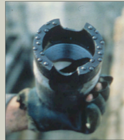
Bit with tungsten carbide bit
