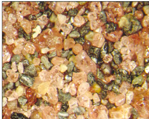
Till heavy mineral concentrate containing abundant orange Fe-rich almandine that may be misidentified as E-garnet
