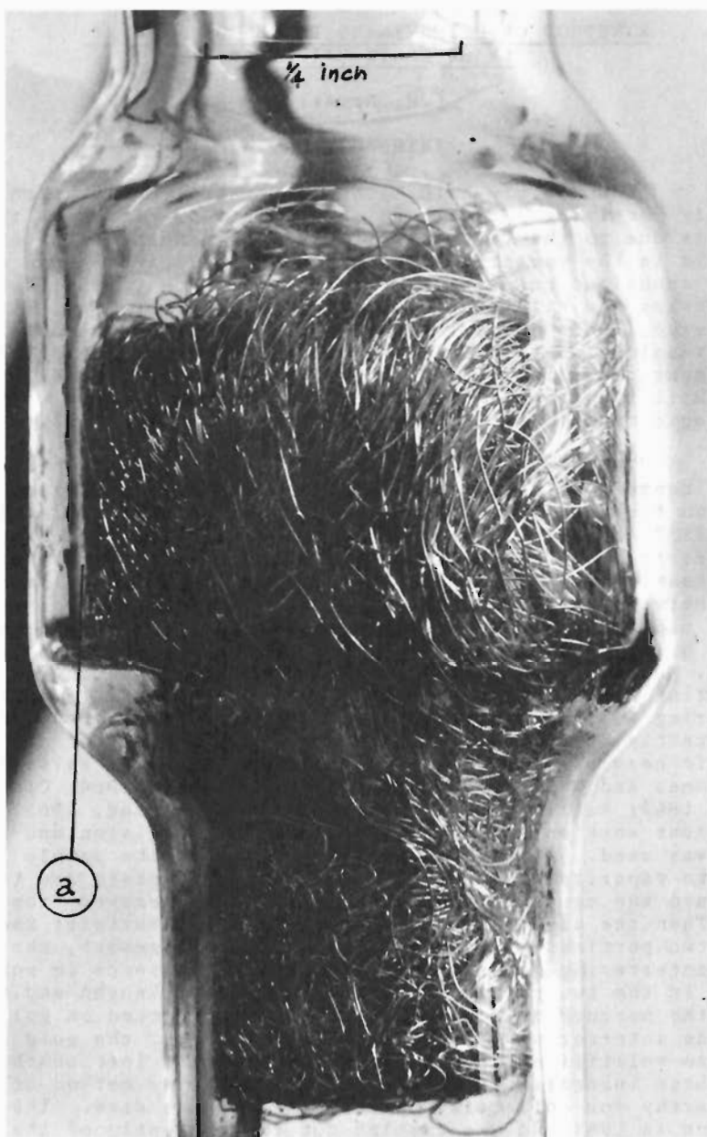
Figure 1. The gold wool collector and emitter of traces of mercury. a: The space produced all around the bulb due to the packing of the gold wool.
