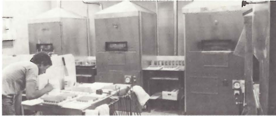
Fire Assaying for precious metals with gravimetric, atomic absorption or neutron activation finish
