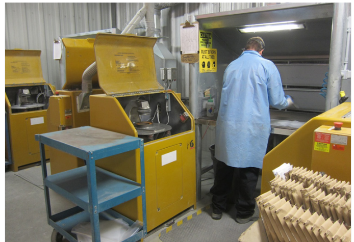
Figure 1. Example of the use of two pulverisers in the sample preparation stream.
