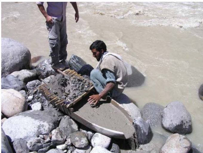
Figure 2: Sluicing of gold along the Gilgitriver in Gilgit area, north Pakistan by the local gold wاهر
