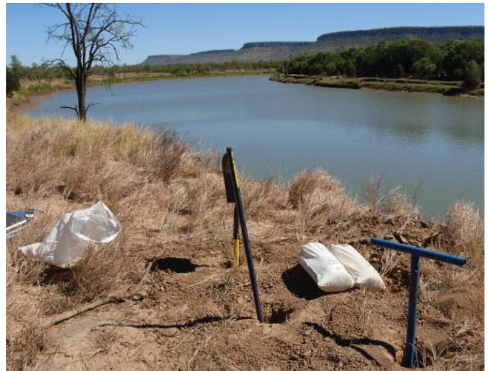
Figure 2. Auger holes drilled to collect BOS samples at a site in the Northern Territory. Note that several auger holes were sampled at each site and combined into the BOS samples to minimise the effect of natural local compositional variability (Photo: Andrew Wygralak, Northern Territory Geological Survey).
