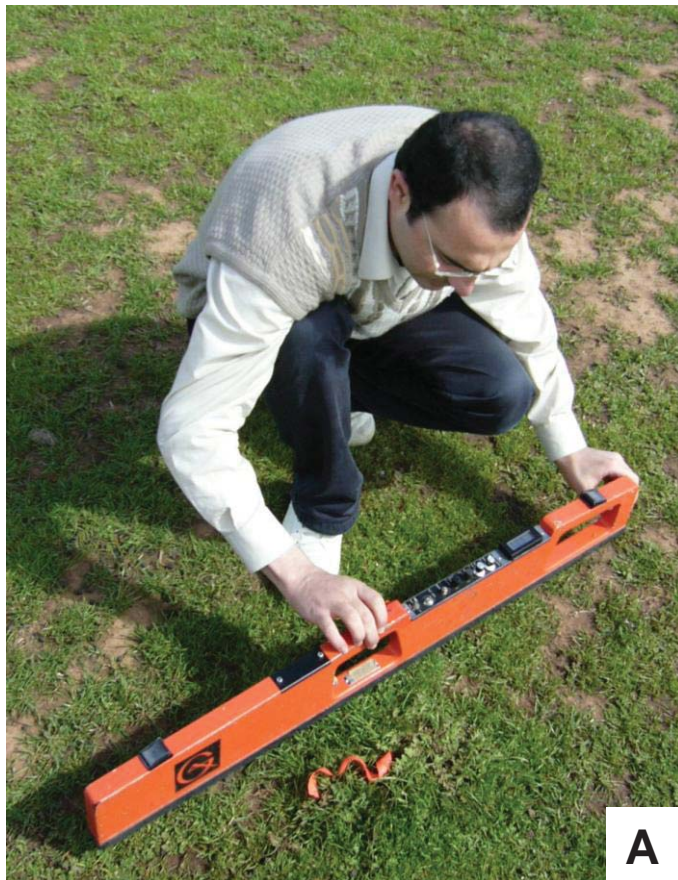
Figure 4. (A) Measurement of shallow EM measurements using a Geonix EM38. (B) Example of typical profiles through the upper 1.5 m of transported regolith at Mandamah. The upper 30 cm is disturbed by ploughing and displays near-neutral pH. Between 30 cm and ~70 cm depth there is carbonate accumulation and the pH is 9 to 9.5. Below 70 cm the regolith displays pH 5 to 6 and Fe mottling.
