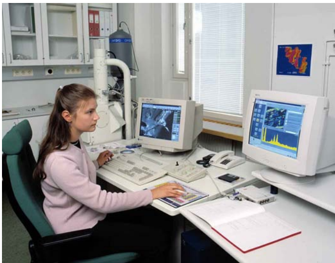
Figure 4. All indicator grains are confirmed by an EDS equipped Jeol JSM-5900LV scanning electron microscope. (Photo: Jari Väättäinen, GTK).
