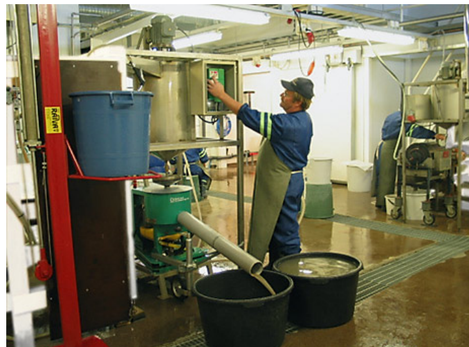
Figure 2. GTK has developed high recovery separation techniques for indicator minerals, including duplicated preconcentration with a modified Knelson concentrator. (Photo: GTK).
