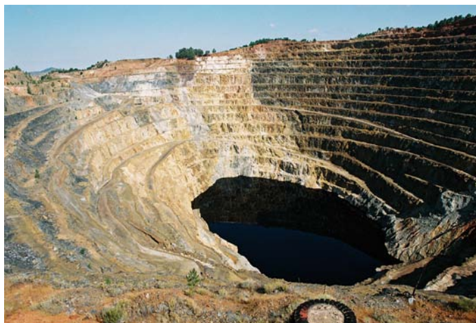
Figure 3. Rio Tinto pit: Corta Atalaya open pit on the San Dionisio VMS lens, Rio Tinto. The base of the pit flooded from 2004 when pumping of the underground workings stopped. (Photo: Tony Christie).
