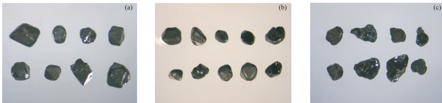
Figure 1. Binocular microscope photographs of representative populations of transported chromite grains derived from specific bedrock lithologies. All grains are of 0.5 to 1.0 mm size. (a) sharp to ragged crystals derived from peridotite; (b) resorbed crystals derived from kimberlite; (c) crystals corroded by lateritic weathering, masking their primary form and paragenesis.
