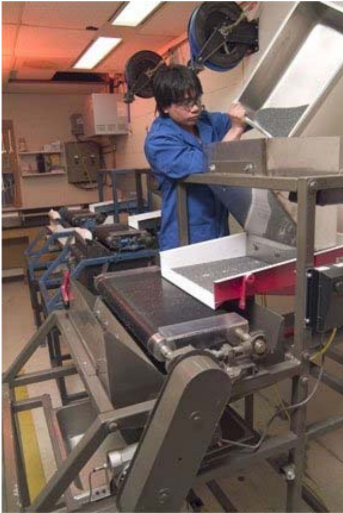
Figure 2. The permroll is used to separate material into paramagnetic and non-magnetic fractions. The paramagnetic fraction is then further processed through heavy liquids prior to picking of kimberlite indicator minerals.
