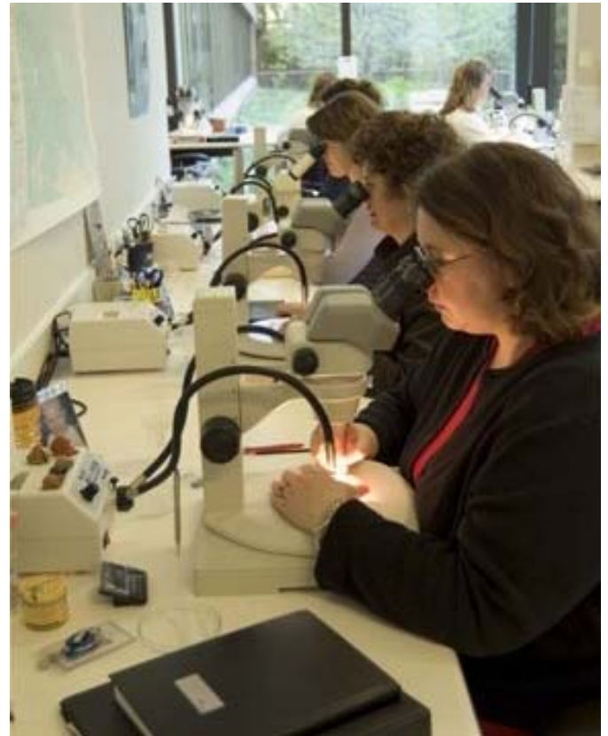
Figure 3. The +0.250-0.500 mm and +0.500-1.00 mm heavy mineral concentrates are observed under a binocular microscope and kimberlite indicator minerals are picked and counted.
