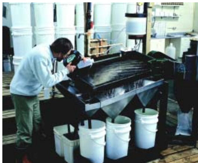
Figure 2 - Heavy mineral preconcentration by tabling, ODM laboratory.
