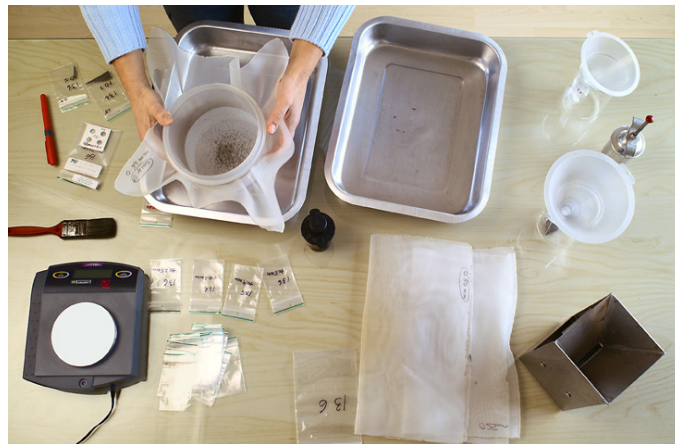
Figure 1. Screening samples into different size fractions before KIM observation.
