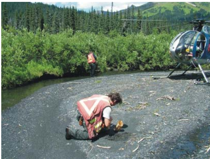
Figure 2. Helicopter supported stream sediment and water sampling in northwestern British Columbia. Roughly 2 kg of fine textured sediment is being collected from a stream bar in the active channel above the current low water level. Extremely high or low energy stream sites are avoided where ever possible so that the sample is representative of the sediment. A 250 ml bulk water sample is also being taken from the stream for later analysis of pH and other elements.
