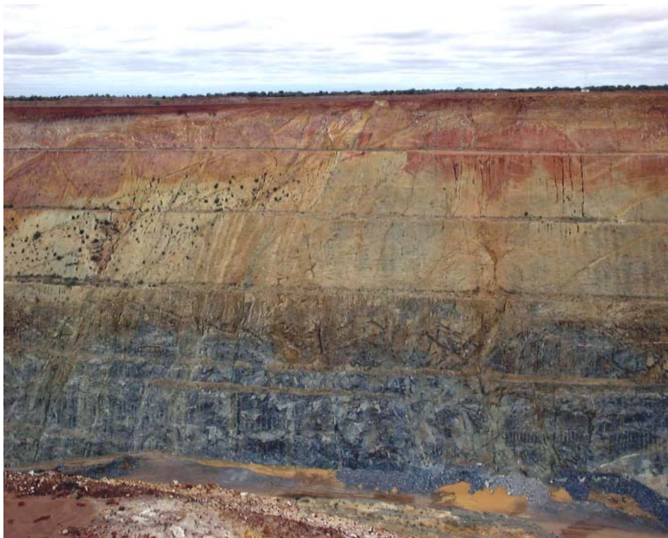
Figure 1. Photograph of typical Yilgarn weathering profile exposed in Darlot open pit (north-eastern Yilgarn). Note flat landscape. Benches height is 20 meters. Rock types are predominantly metadolerite. Profile shows thin “harpanized” soil cover (1-3 meters), mottled lake clays (only at far left in profile, thickening to about 40 meters out of field of view), residual upper saprolite (red and purple colours extending irregularly to about 30 meters, but much deeper on structures), lower saprolite (yellow and, grey-green colours, extending to about 60 meters), saprock transition (irregular zone about 5 meters wide just below 60 meter bench), and fresh rock at about 65 meters to base of pit at around 100 meters below surface.
