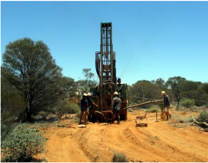
Figure 4: Photograph of typical RAB rig (view from rear) showing sample delivery through “stuffing box” at collar along flexible tube under pressure to cyclone (at right) for collection. Note hard hats and safety boots for all personnel- a recent safety change to replace caps and thongs!
