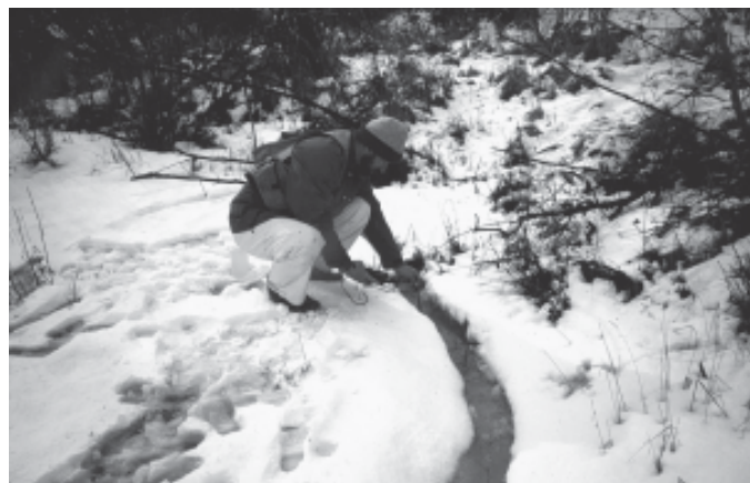
Figure 1. Eppinger collecting water pH from stream below the Nabesna mill tailings pile during spring breakup in April, 1997. Water temperature 0° C, pH 2.8, conductivity 1600 \mu S/cm. Same site during the summer months had pH 7.2 and conductivity 580 \mu S/cm, demonstrating importance of snowmelt and seasonality to water composition.
