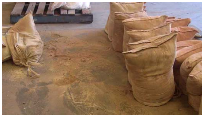
Figure 1- Dry samples received by the laboratory in calico bags may split and leak drill cuttings from one sample to the next during shipment. Spilled material is evident by the footprints on the floor.
