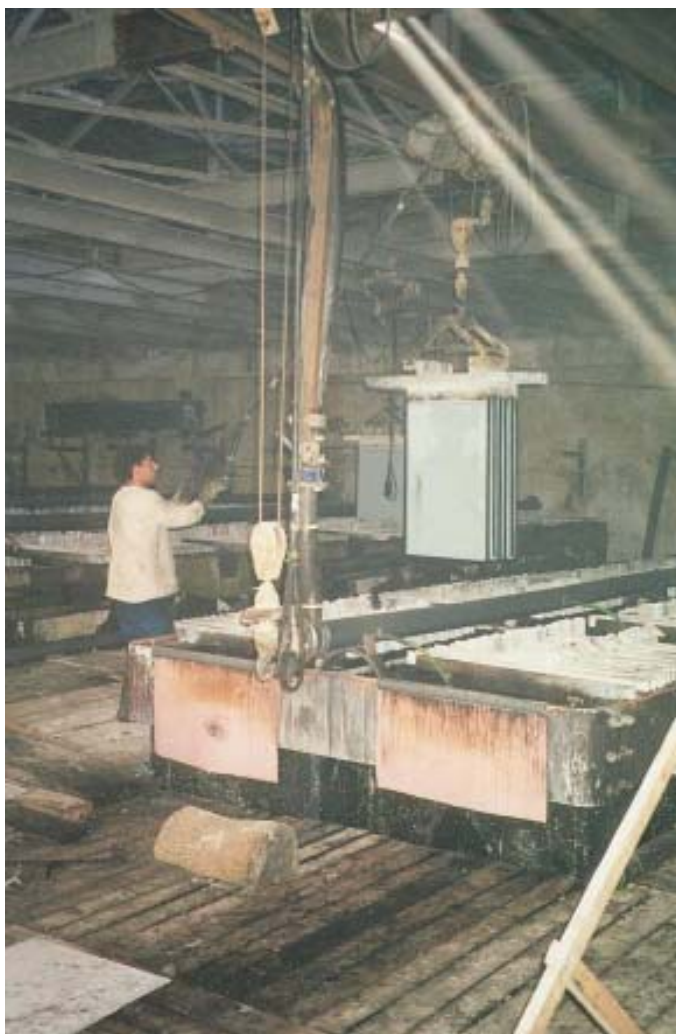
Figure 4: Traditional zinc tankhouse where metal is recovered by electrolysis. KCM, Bulgaria.
