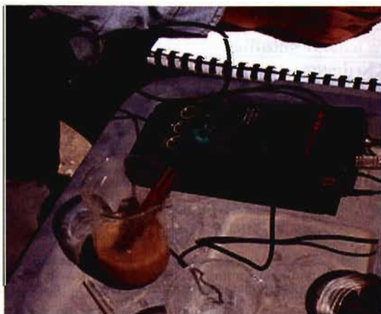
Plate 1: Field Portable pH meter measuring surface soil pH, Atacama desert.
