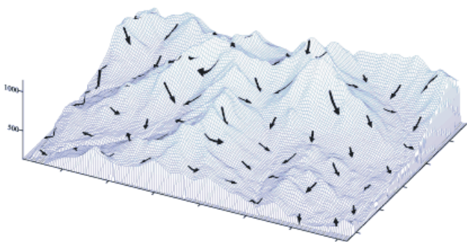
Figure 2: Topographic Wire Frame with Slope Vectors
