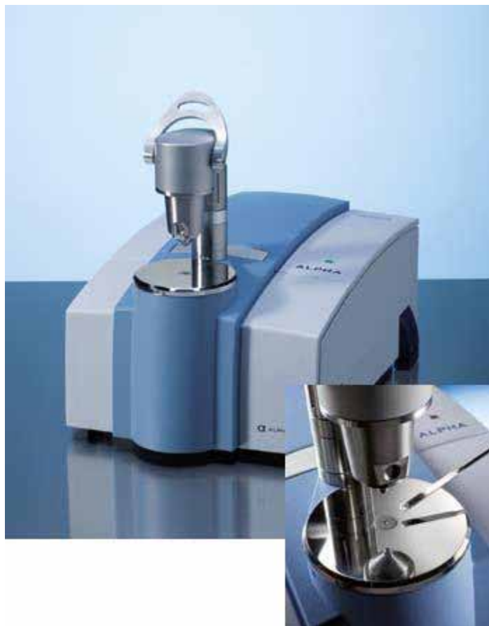
Figure 1. Bruker Alpha FTIR fitted with ATR unit inset showing sample plate (image courtesy of Bruker) used in the quantitative determination of common rock forming minerals.
