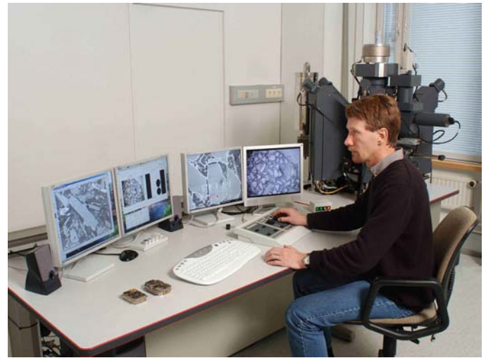
Figure 6. Cameca SX50 microprobe offers rapid and cost-effective quantitative analysis of indicator minerals. (Photo: Jari Väättäinen, GTK).
