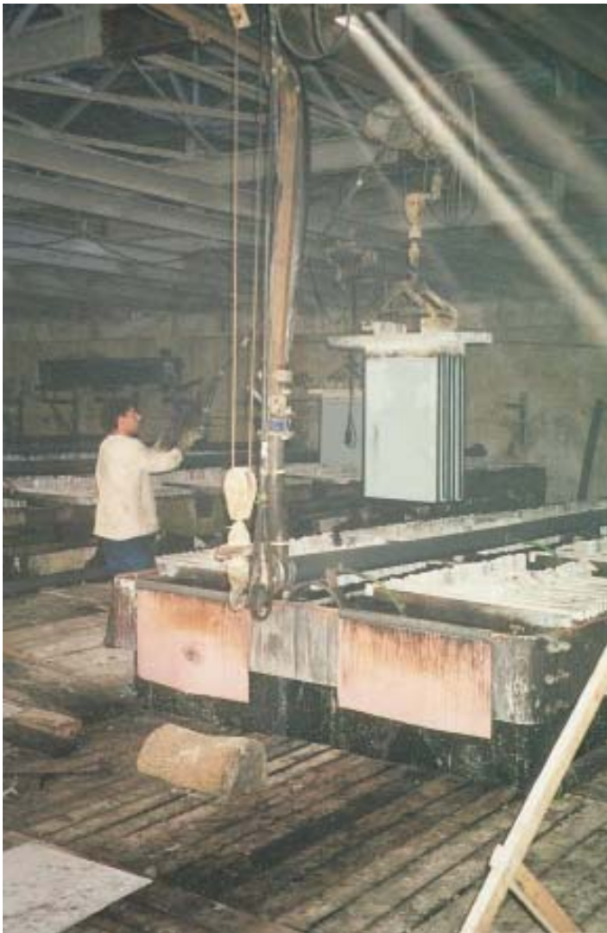
Figure 4: Traditional zinc tankhouse where metal is recovered by electrolysis. KCM, Bulgaria.
