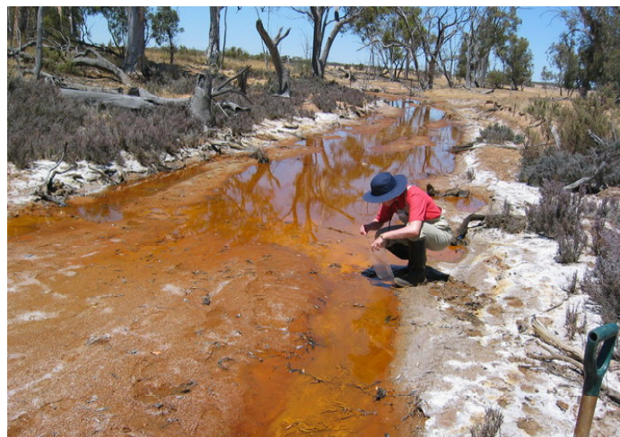
Figure 9. Iron oxy-hydroxide minerals covering the base of a stream, note also the abundance of salt efflorescences adjacent to the stream caused by evaporation of capillary water. The efflorescences are generally present during summer months but are washed into the stream during rainfall periods, producing a pulse of increased salinity.
