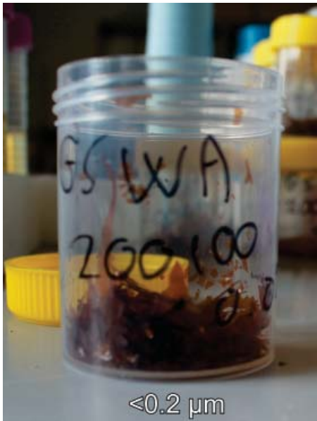
Figure 4. Using centrifugation to separate the <0.2 μm (or 200 nm) size fraction results in dry films (dark red material) of soil weighing between 0.1 and 0.5 g that were then subject to aqua regia digestion.
